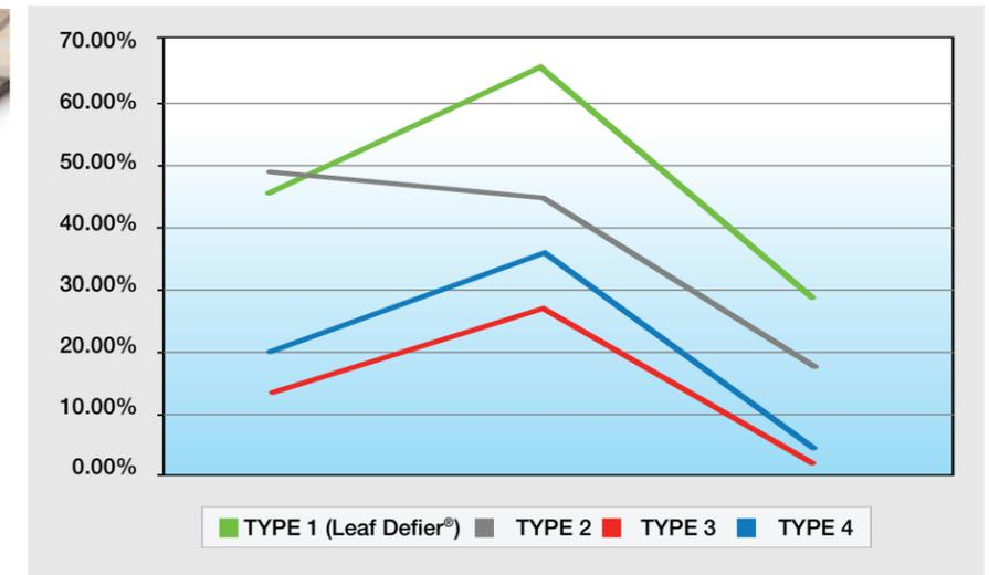
In short the force needed to deflect the XENON exposed "multi-polymer" fusion coated product (TYPE 1 [Leaf Defier®]) by 50 % after 4500 hours of exposure (equivalent to five years UV exposure) was 28.44 % of the force needed to deflect the unexposed material. All other materials show significantly inferior performance at the maximum exposure time of 4500 hours.
