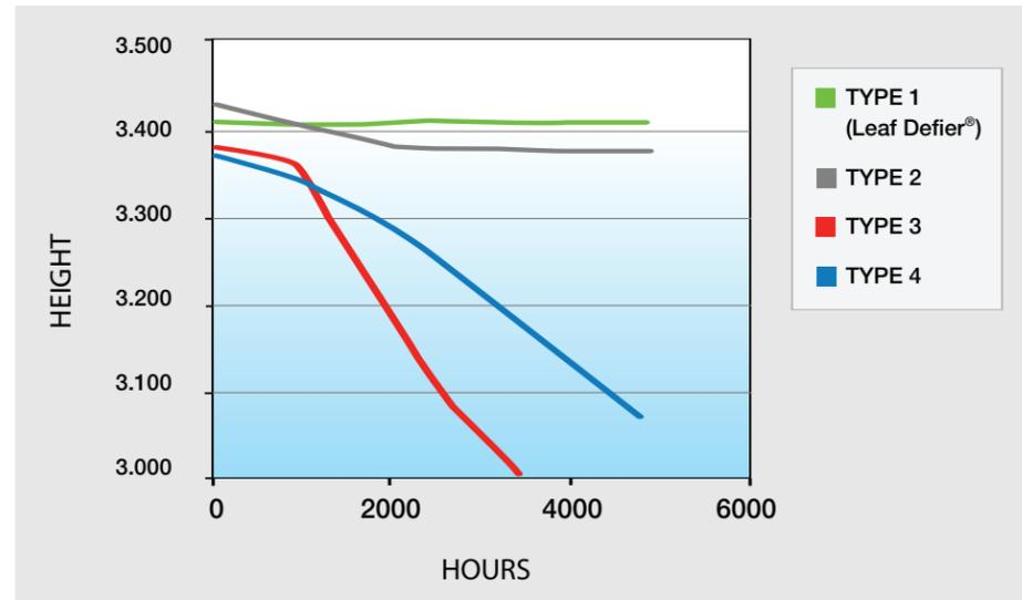
As the above table indicates, the % loss or exposed surface degradation was minimal with the TYPE 1 (Leaf Defier®) "multi-polymer" fusion coated product available from Leaf Defier®. The surface degradation with this "multi-polymer" material is LESS THAN one tenth of 1 % as compared to significant losses in surface character with the other materials tested.
